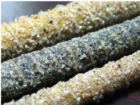
Figure 5.14 – FRP reinforcement with sand coat for bond. ( http://www.b-composites.net/245.html )
