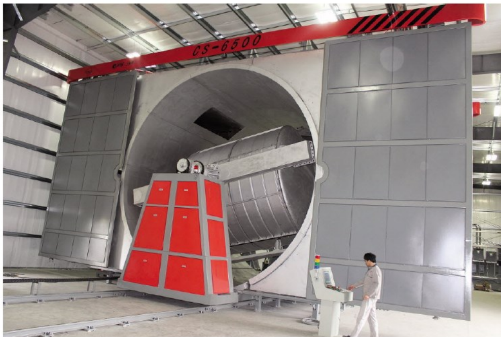
Figure 5.3. The gigantic rotomoulding machine measures 6.5 metres in diameter, 27 metres in length, 17 metres in width and 8 meters in height. [from Ref. 5]
