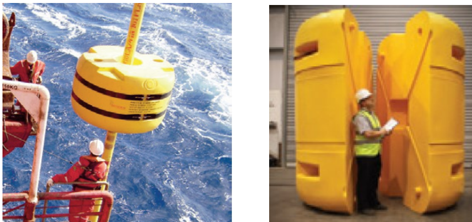
Figure 5.4. Rotomoulded polymer buoyancy modules for oil and gas risers generally consist of an internal clamping system and syntactic foam buoyancy elements. The buoyancy elements are supplied in two halves incorporating a moulded internal recess that is configured to transfer the forces from the buoyancy to the clamp and subsequently the riser. [from Ref. 18, Balmoral Offshore Engineering]
