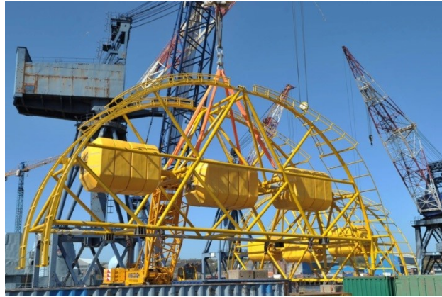
Figure 5.25. Composite Mid-Water Arch from Buoyancy Units
