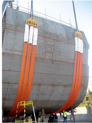
Figure 5.8. Extreema Slings used to distribute loading [from Ref 6]
