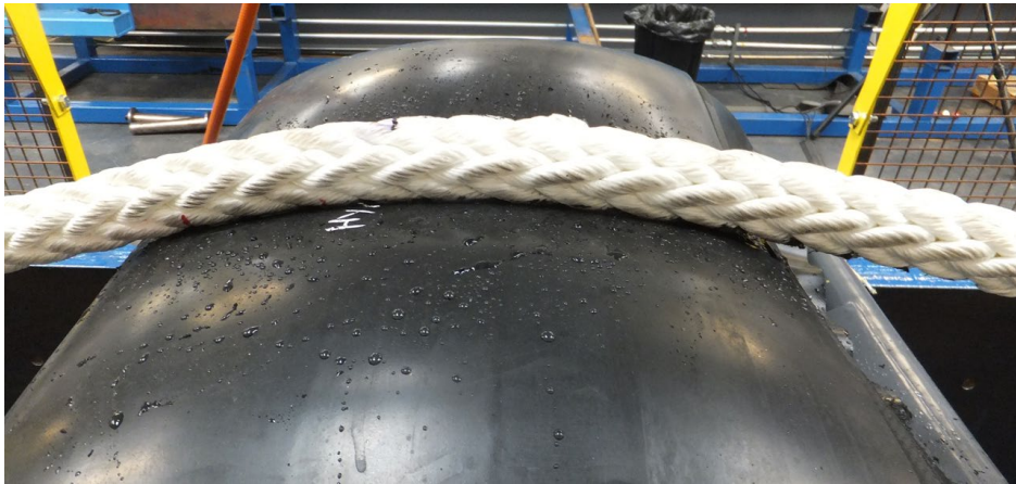
Rope on Pillow Abrasion – 5 Candidate Elastomers
