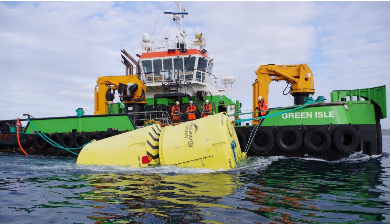
Figure 11: Waveswing under tow alongside the Green Isle multicat work-boat
