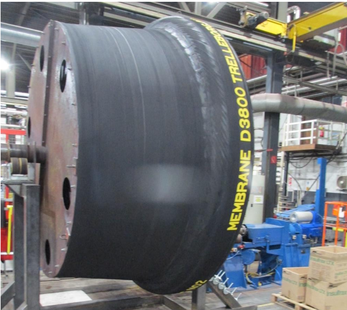
Figure 3: Rolling seal on former in Trelleborg factory
