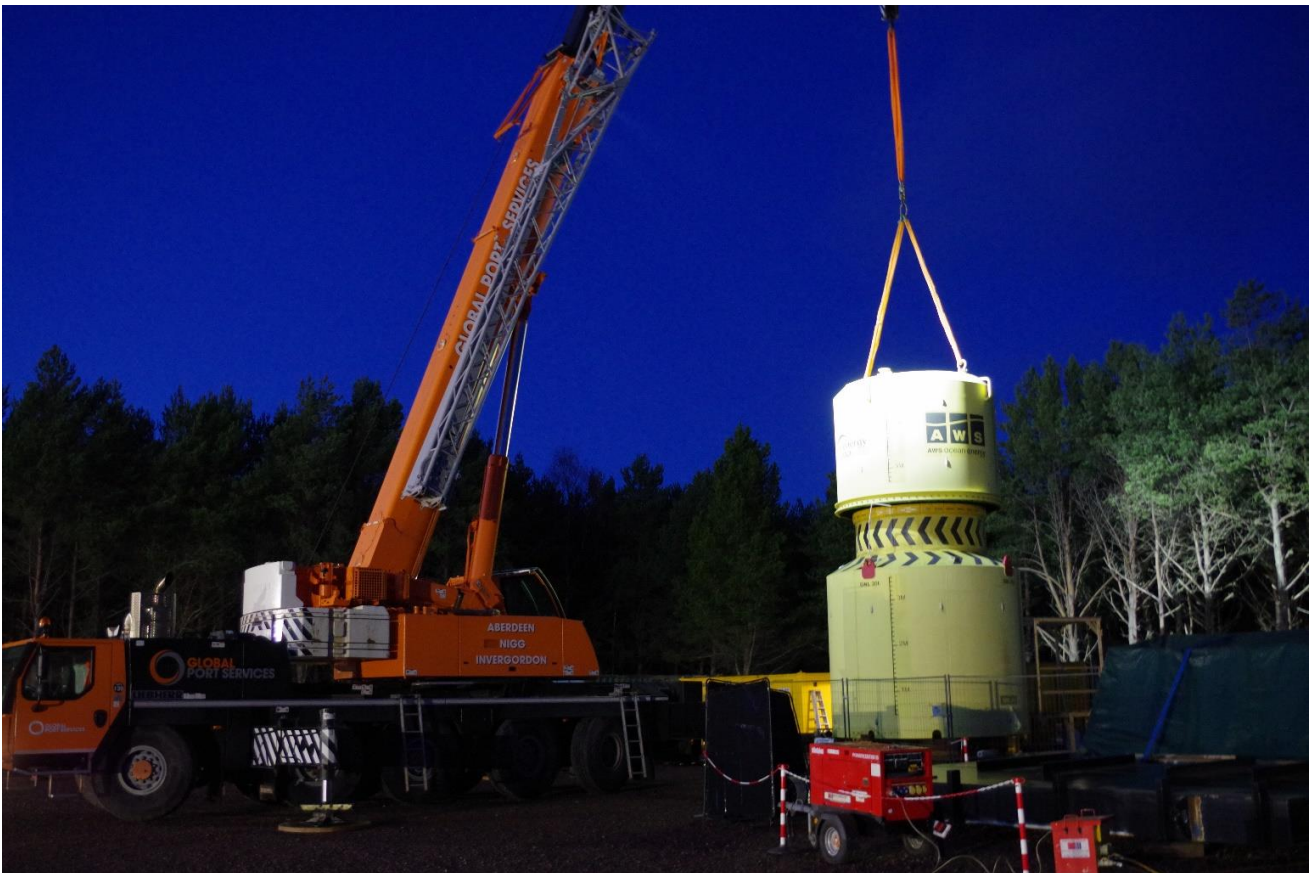
Figure 7: Cyclic testing of Waveswing at crane yard in Muir of Ord
