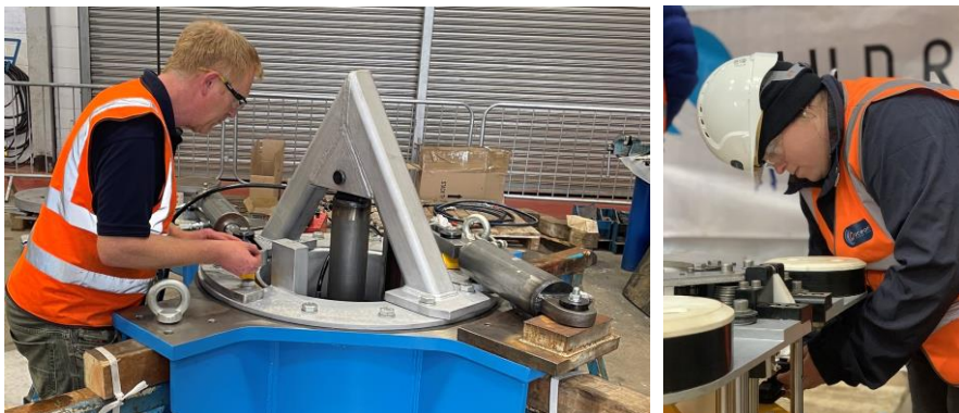
Figure 2: Subsystem tests (left) of the mechanical latching system and (right) of the wet mate capping system.
