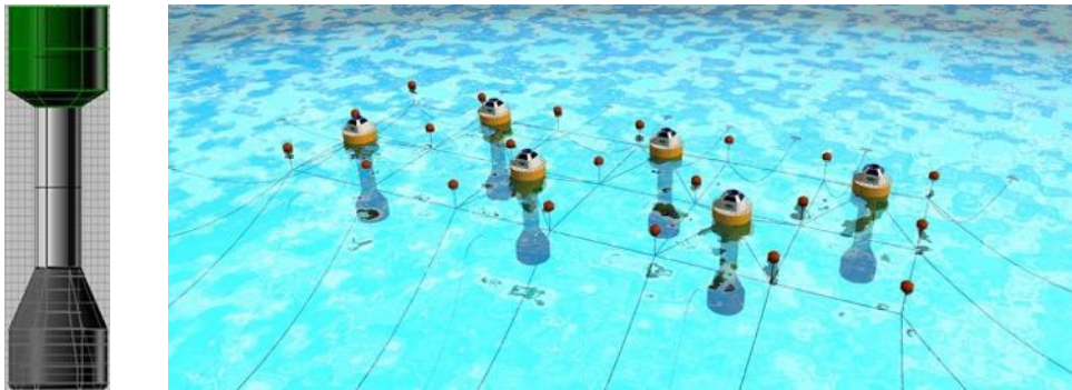
Figure 1.6: left - MARMOK-A-5 hull design; right - Artistic representation of an array.
