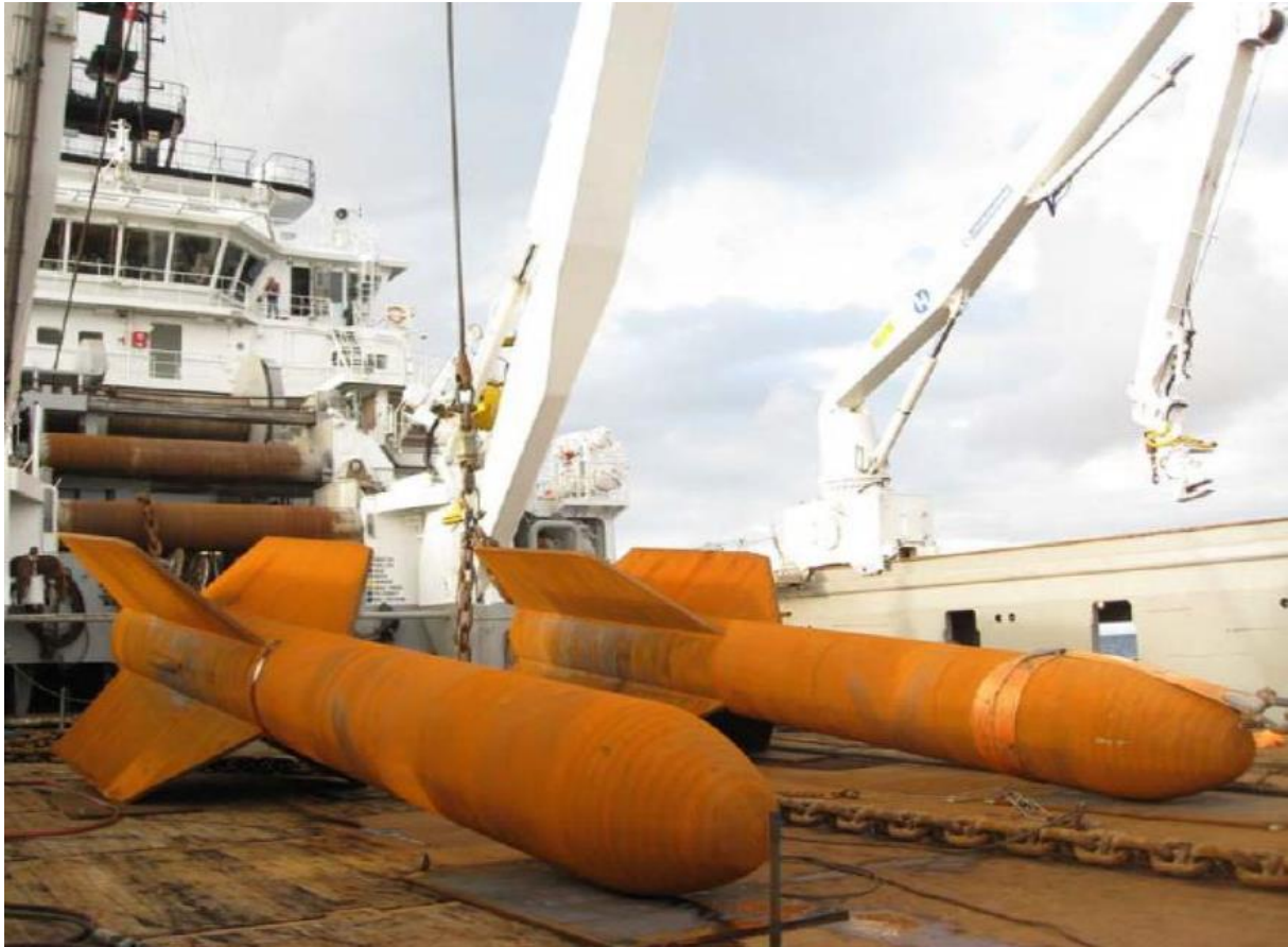
Figure 66: Deep penetration (torpedo) anchors for cohesive sediment sites (source: Deep Sea Anchors).
