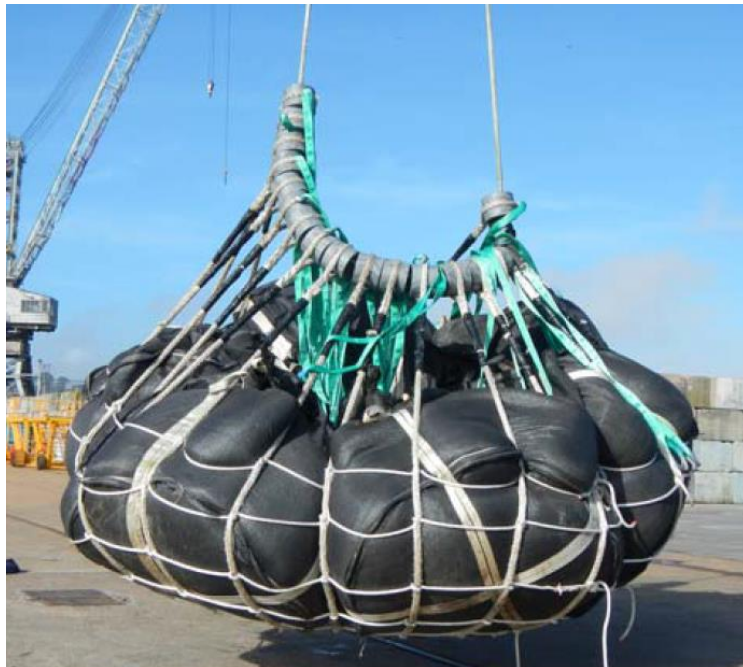
Figure 20: Early anchor bag prototype undergoing lift trials (source: TTI).
