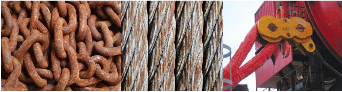
Figure 4: Examples of metallic mooring components: (left) Mooring chain (source: www.pexels.com ), (centre) wire rope (source: www.pexels.com ) and (right) Steel connector with 1700T break load polyester rope (source: TTI)
