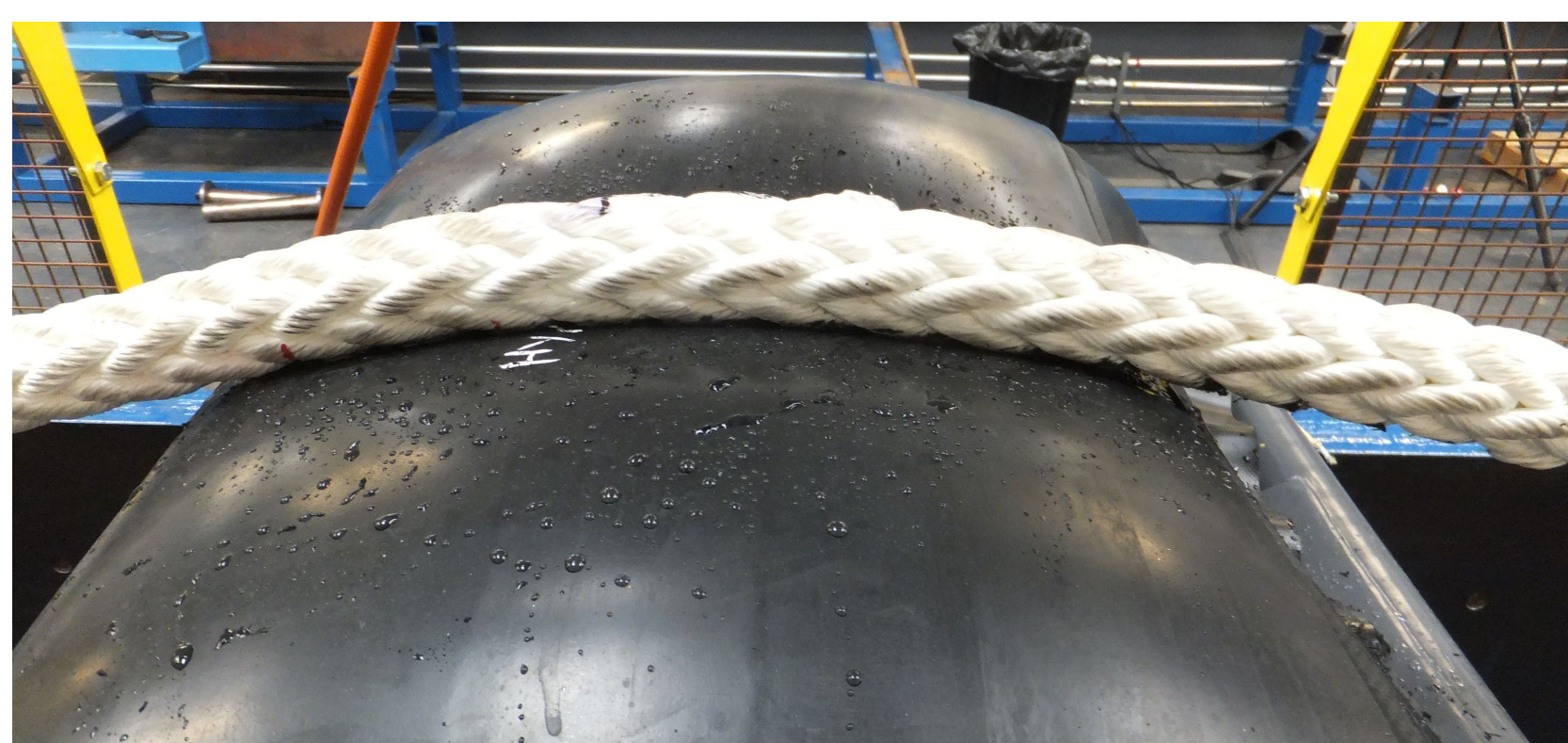
Full-scale rope abrasion tests on inflated pillows (5 candidate membranes)
