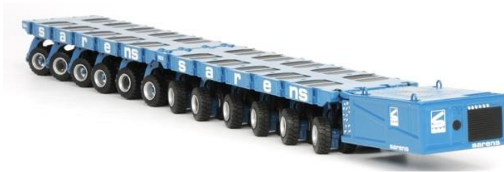
Figure 23. Two Sarens 6 axle SPMT units with powerpack
