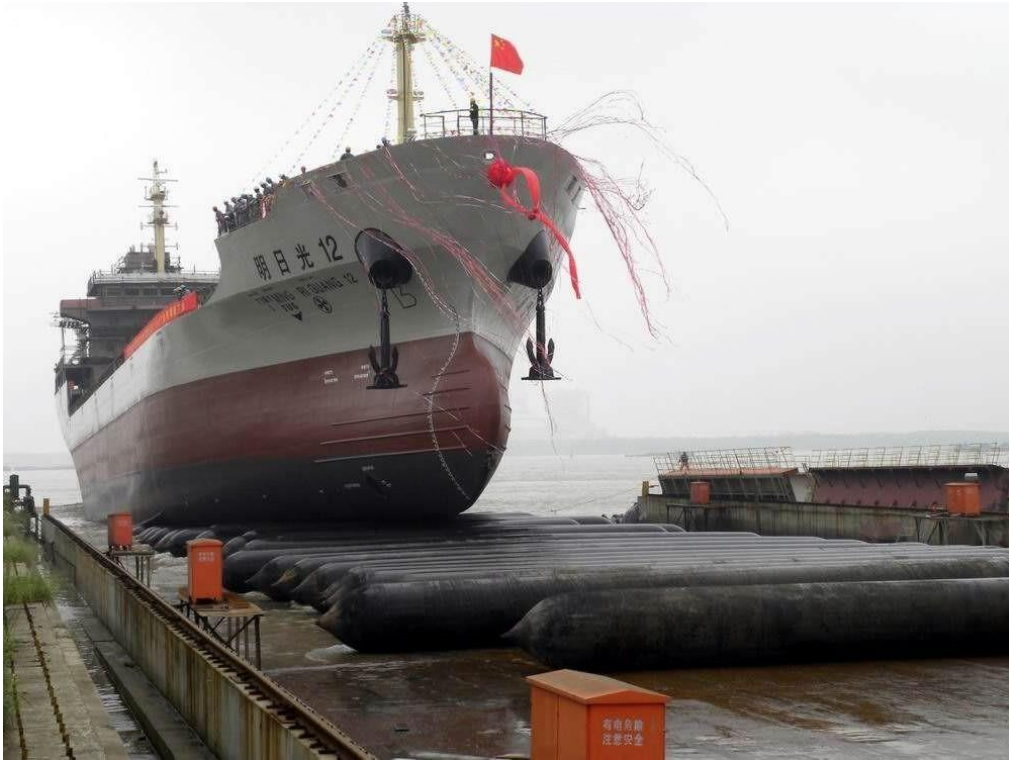
Figure 24. Ship launch on slipway using compressed air roller bags
