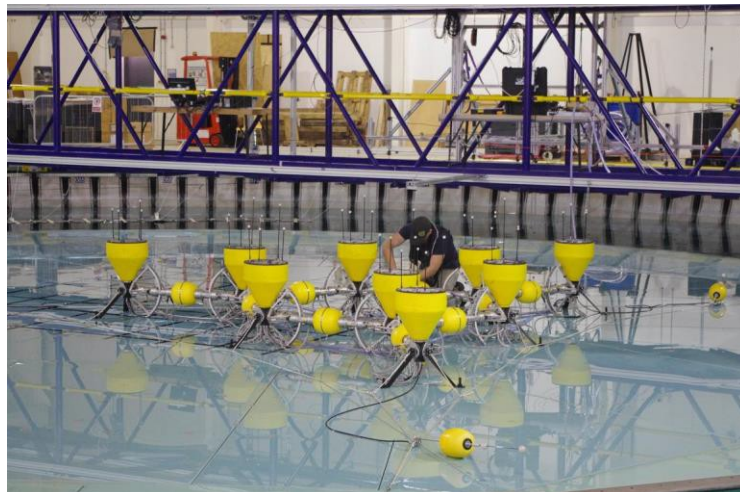
Figure 4: 1Hex model on Flowave's raisable floor
