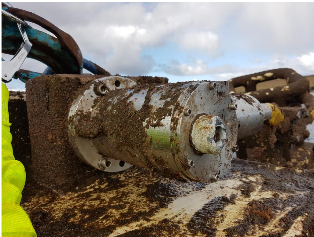
NovaCAN: operational MEC dry-mate connector variant with typical biofouling
