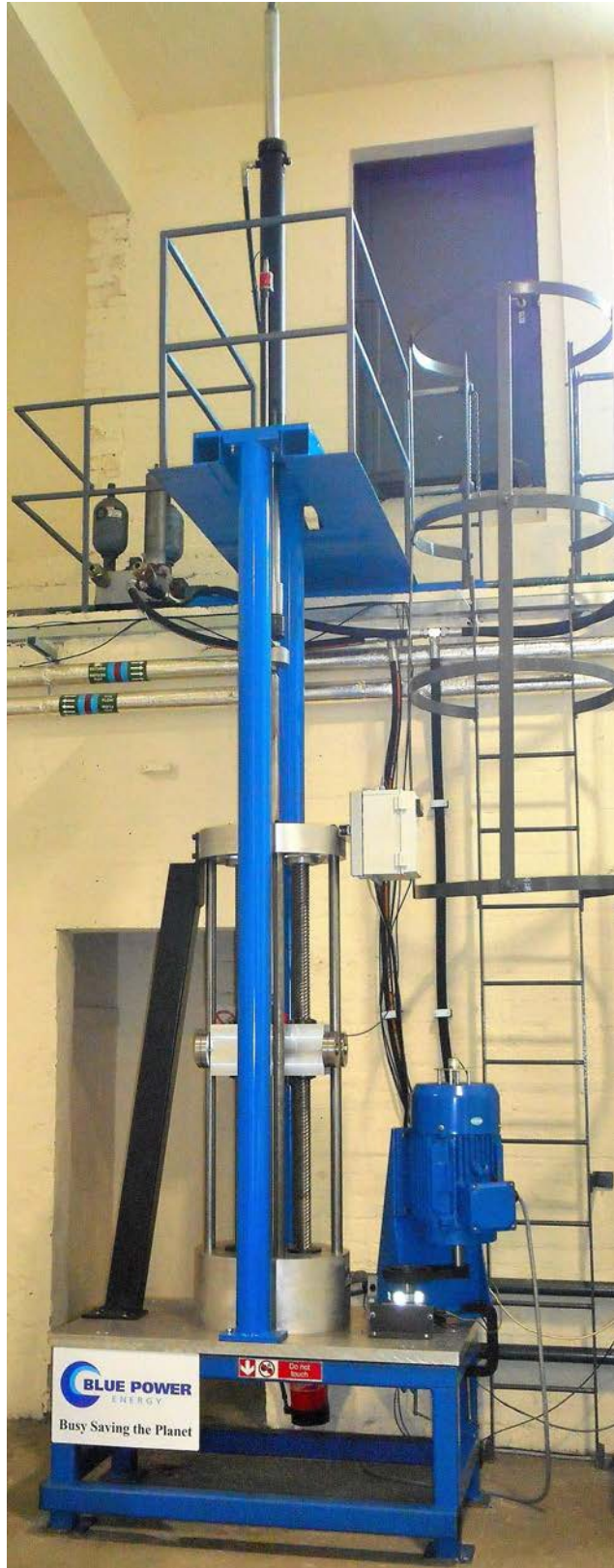
Figure 3 Bespoke Hydraulic Test Rig with Blue Power PTO
