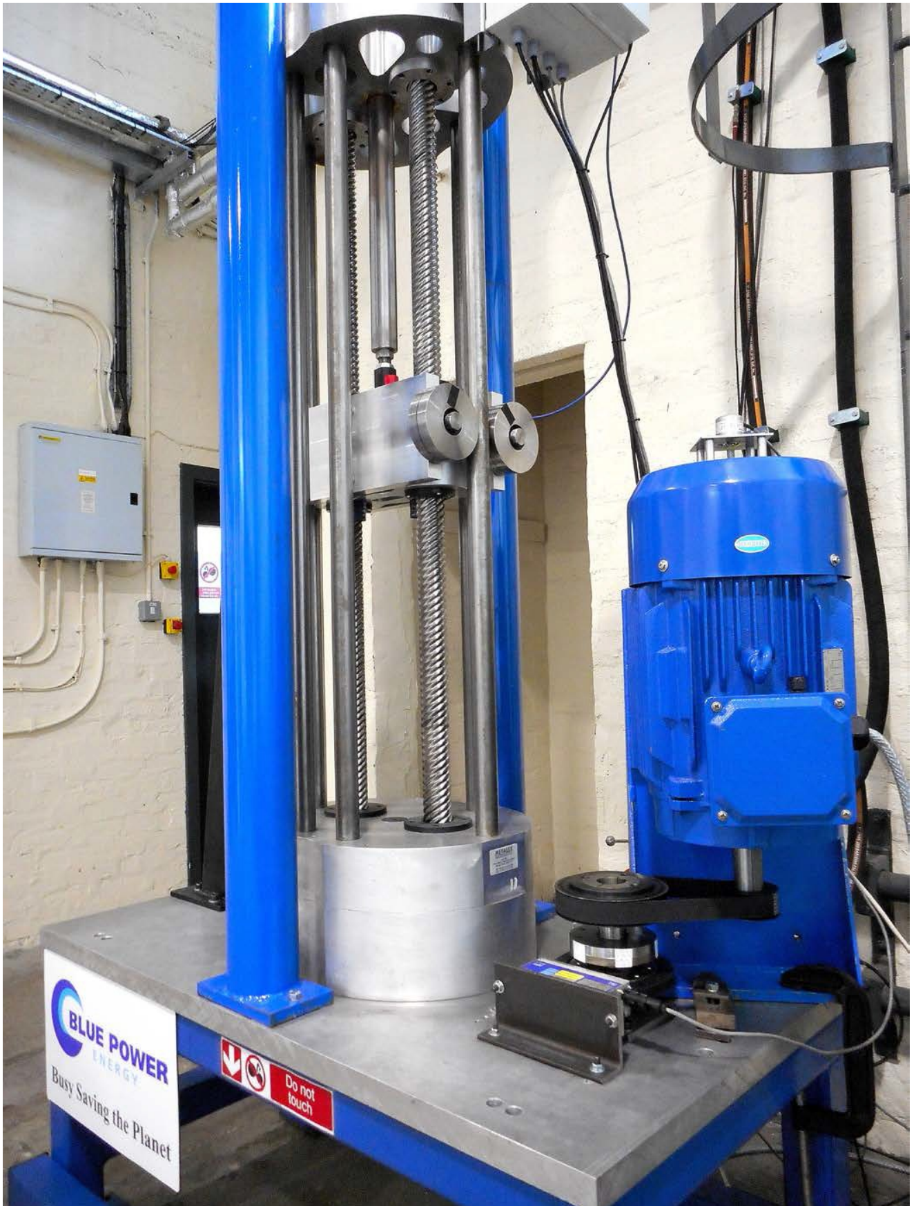
Figure 2 As-Built Blue Power PTO
