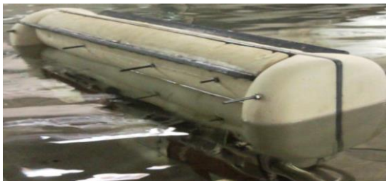
(b) Protruding strips on the front & back edge
