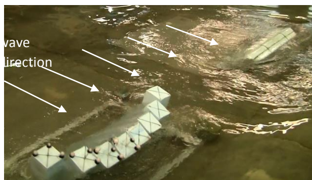
Figure 67. Comparison of an 8-module WEC (left) alongside a rigid flap of comparable width.
