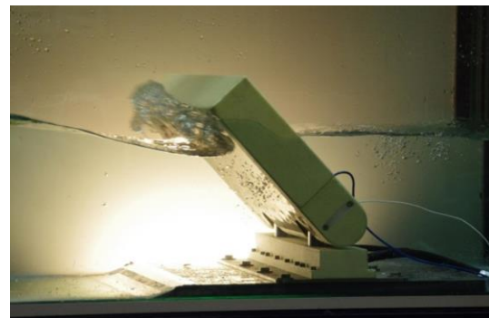
Figure 52. Experimental flap model in 2D tests
