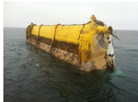
Figure 46. Bio-fouling on Oyster800 after a nine month period of submersion prior to first operation
