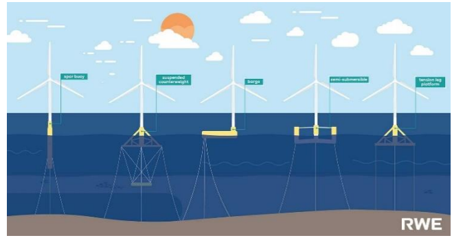
Fig. 2. Supporting platform types being explored by floating offshore wind project developers (Source: https://www.rwe.com/en/research-and-development/wind-power/floating-offshore-wind/floating-wind-education/ ).
