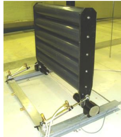
Figure 15. Double-acting hydraulic cylinder attached to a flap model.
