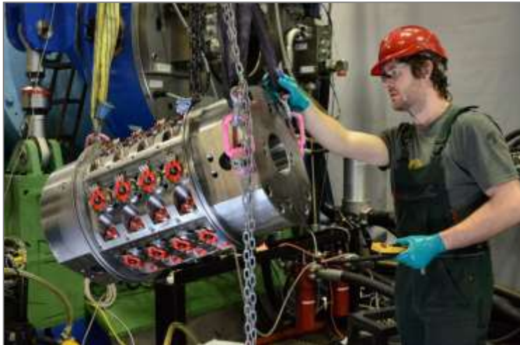
Dual service pump-motor
