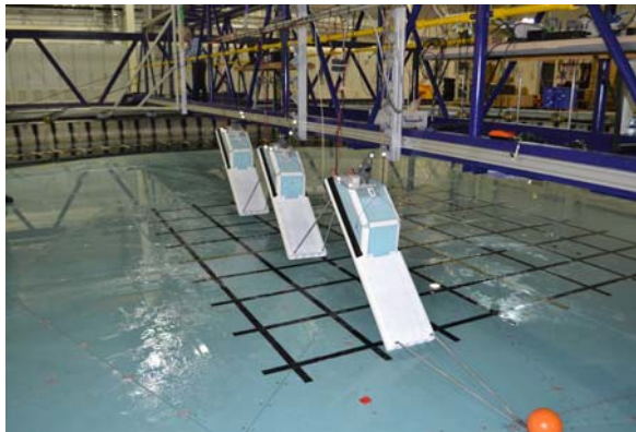
Figure 1.2: WaveTrain array suspended prior to immersion in the FloWave tank (Photograph copyright Joules)
