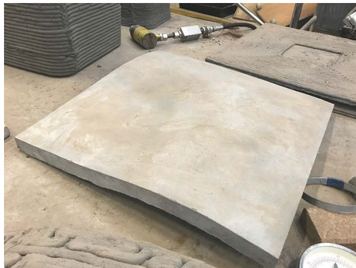
Figure 1 Sample 3D printed concrete slab sections indicating layered construction and intricate slab curvature (courtesy of Loughborough University 3DCP Centre)
