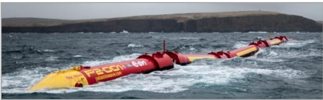
Pelamis with Quantised hydraulic PTO
