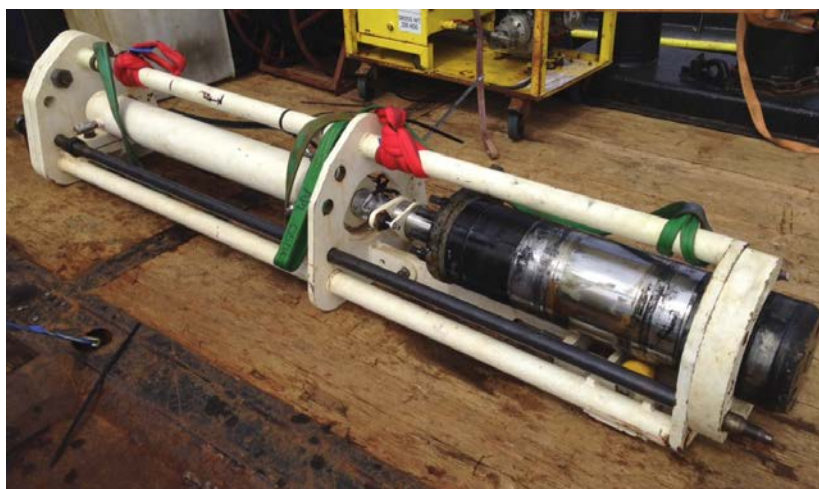
Figure 5 - Bondura Bolt, secured within the bespoke Bondura Bolt removal tool
