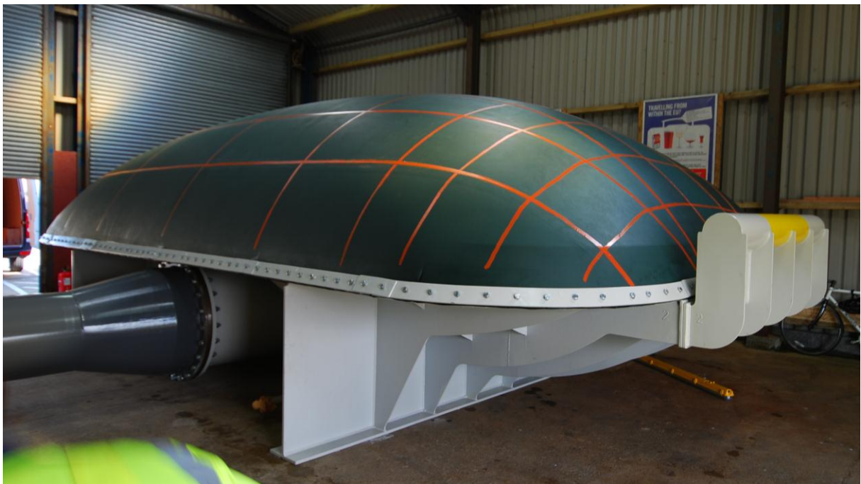
Figure 7: Half-scale cassette under test - diaphragm fully inflated
