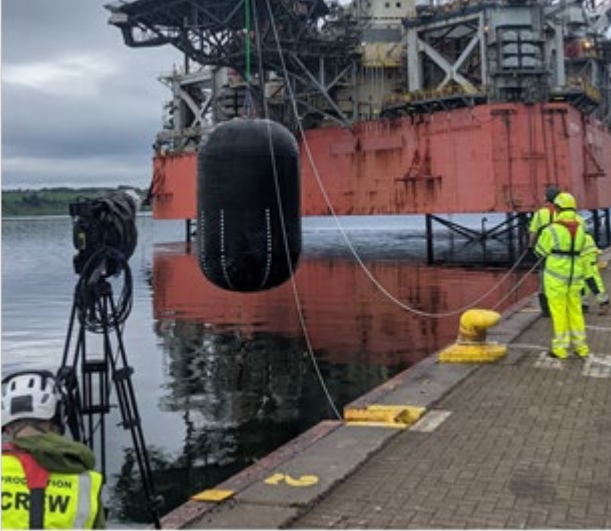
Figure 12 Heriot Watt University's biofouling test rig with NetBuoy candidate and control materials (pre-deployment)
