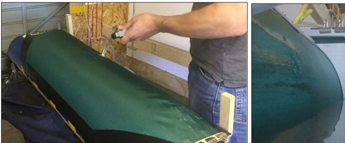
Figure 4: functional testing of the MASIV system; (left) air tightness testing prior to test and (right), measurement and recording of inflated shape in the water
