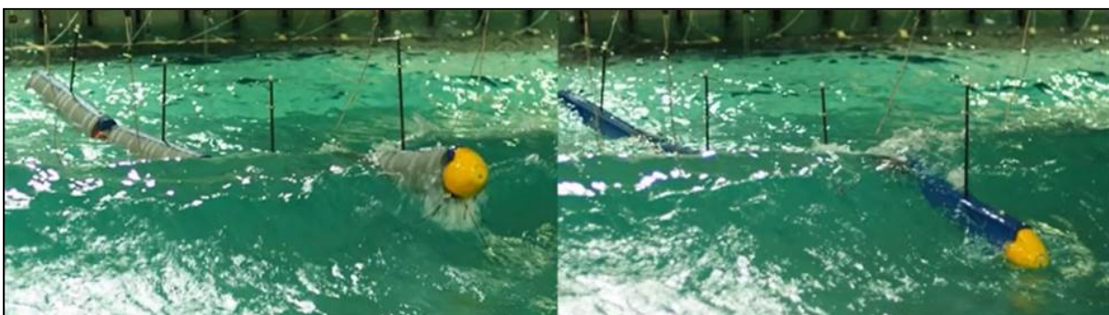
Figure 2: Captures from synchronised video of HV & LV models in Quocean defined 'steep' sea state at wave steepness limit ( H_s = 7.5\text{m} , T_e = 9\text{s} ). Capture from extreme wave section ( H_{\text{max}} = 14.3\text{m} )
