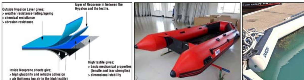
Figure 4 (left-to-right): Layered construction of fabric material commonly used in many marine applications already available on the market, example use in rigid inflatable boat, example use in quayside fender systems.
