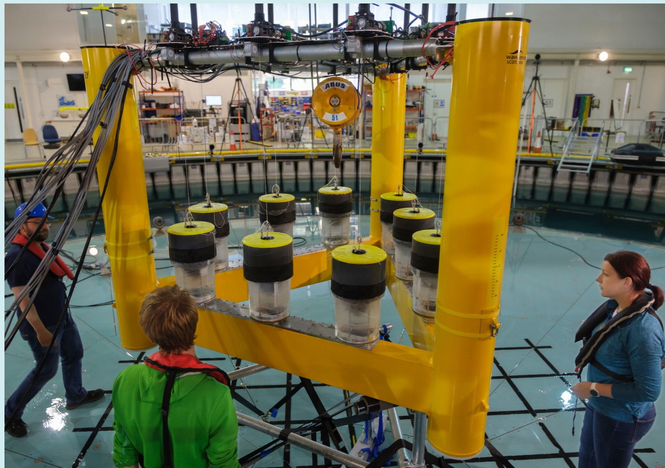
Testing multiple WECs on a floating-wind-scale semi-submersible platform at FloWave (Credit: Wave Energy Scotland)
