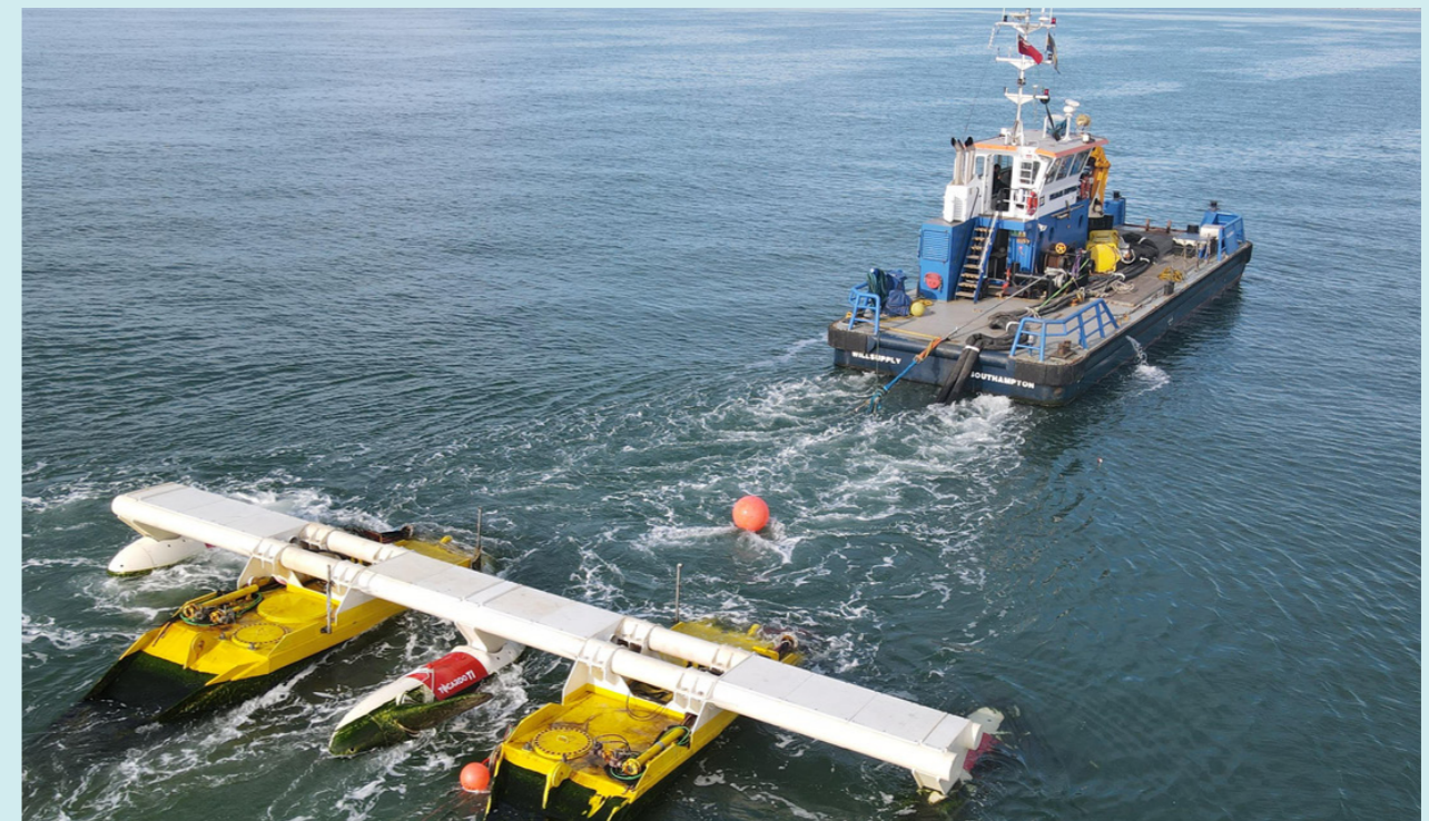
QED Naval's Subhub being towed to Langston Harbour for testing (Credit: QED Naval)
