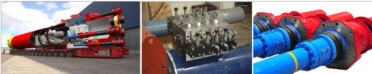
Pelamis switched state PTO. Left: complete system; Centre: chamber switching valve matrix mounted directly to hydraulic ram; Right: multi-chamber hydraulic rams.
