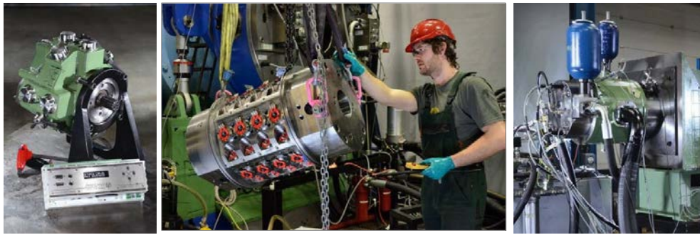
Artemis Digital Displacement® hydraulic machines. Left: 'E-dyn 96' 12-cylinder ~75kW industrial pump with controller; Centre: 'Q40' 24-cylinder pump-motor (DDPM) modified for the WES project to provide two independent 'services'; The Q40 DDPM mounted as set up for the Stage lab tests
