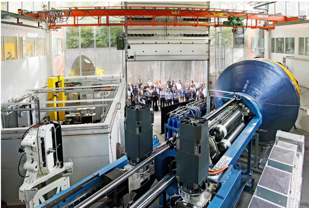
Figure 6 Stage 3 WEC in CorPower dry Hardware-in-the-loop testing facility, Stockholm (Sweden)
